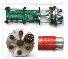
The FDL-Multi is a customized data logger for the operation of various sensors on a bottom station.
